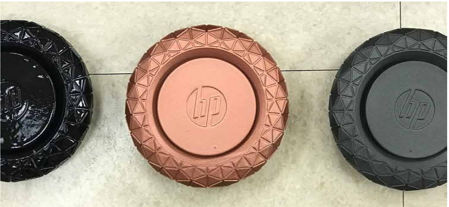
Above : MJF parts dyed and painted various colors and sheens.
