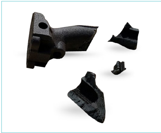
Raw part after impact test
