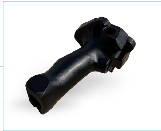
Post-Processed part after impact test
